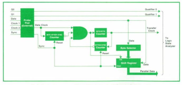
Fig. 2. Simplified block diagram of Model 10254A Serial-to-Parallel Converter. Serial-to-parallel conversion occurs in the shift register. The other blocks control the timing and direction of shift register loading and the timing of data transfer to the logic state analyzer.
