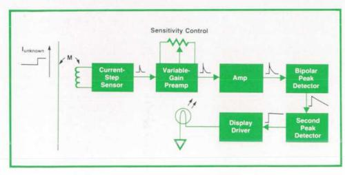
Fig. 5. 547A Current Tracer block diagram. Current-step sensor detects current steps as small as 1mA and rejects magnetic flux that is not directly beneath the tracer's tip.
