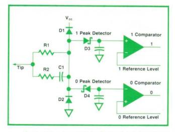
Fig. 2. 545A front-end has two fast peak detectors and two relatively slow, low-input-current comparators. The circuit can withstand accidental overloads of  $\pm 120V$  continuous and  $\pm 250V$  for 15 seconds.
