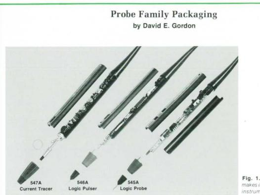
The problem was to design a second generation probe packaging system for three new logic test instruments, accommodating 100% more circuit area with minimal instrument size increase, 200% more heat dissipation, and electromagnetic shielding. The amount to be spent for tooling was strictly limited. It was desirable that all parts be inexpensive, easy to assemble and service, and highly reliable.
