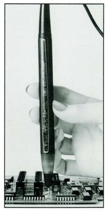
Fig. 1. Model 546A Logic Pulser provides single pulses, pulse bursts, and pulse trains that automatically drive a digital circuit node to its opposite state.
