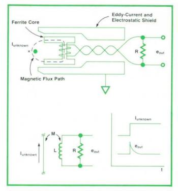
Fig. 6. Construction and equivalent circuit of the currentstep sensor, which acts like a current transformer. For each current step the sensor produces a voltage impulse at its output.
