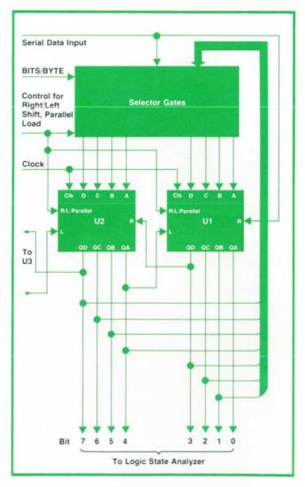
Fig. 3. Block diagram of part of the bidirectional shift register. U1 and U2 are commercial IC 4-bit shift registers (U3 is the next IC in the 16-bit shift register chain). The selector gates enable serial data to be loaded through any bit position during right-shift operation (see text).
