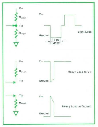
Fig. 5. Typical 546A output waveforms under various loads.
