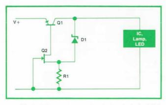
Fig. 3. Power supply protection circuit protects the 545A's single integrated circuit, its tip lamp, and its latch LED against overvoltage and reverse voltage to ±25V.
