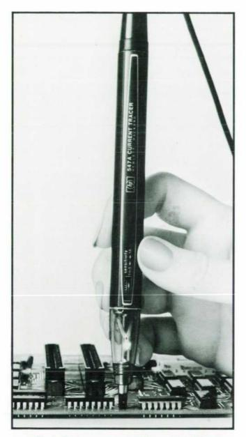
Fig. 1. The lamp near the tip of the new Model 547A Current Tracer varies in brightness according to the relative magnitude of the current steps occurring near its tip. By observing how the lamp's brightness changes as the tracer is moved along the conductors the user can follow the flow of current.
