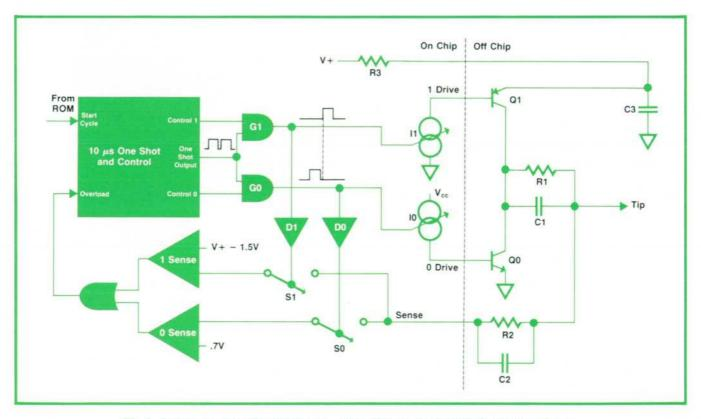
Fig. 4. Functional schematic of 546A output stage. The circuit automatically delivers pulses of the proper polarity, voltage, width, and transition time to override the logic node at the pulser's tip.
