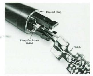
**Fig.3.** Ground ring provides a ground path from the bottom of the printed circuit board to the end of the extrusion shown in Fig. 2. Crimp-on strain relief pulls back into a cavity and locks the cable into place. Notches in the printed circuit board snap into the rear plastic support for structural ridigity.
