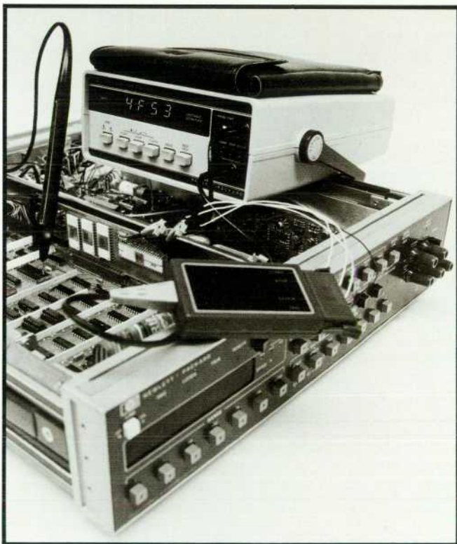
Fig. 7. Model 3455A System Voltmeter is the first HP instrument designed for troubleshooting with the 5004A Signature Analyzer.
