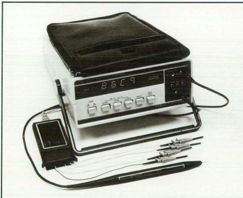
Fig. 1. Model 5004A Signature Analyzer is a new tool for field-troubleshooting of digital circuits to the component level. (The circuits must be designed for signature analysis and must have built-in stimulus.) The 5004A gets start, stop, and clock inputs via its pod, shown here in the foreground, and data inputs via its data probe, which doubles as a logic probe.
