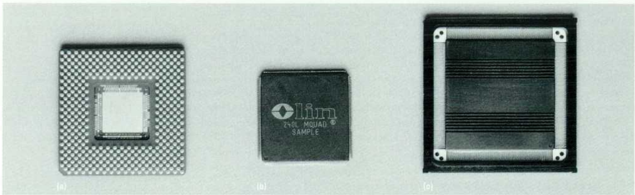
Fig. 2.* (a) 432-pin ceramic pin grid array (432-CPGA). (b) A 240-pin MQUAD and (c) a 304-pin MQUAD.
