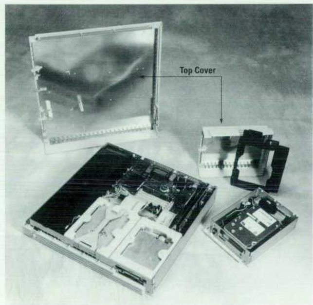
Fig. 2. The Model 712 workstation and hard disk peripheral with top covers disassembled.
