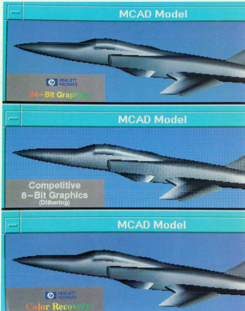
Fig. 1. A true color image and its dithered representations. (a) True color 24-bit image. (b) Typical eight-bit graphics dithered image. (c) An HP Color Recovery dithered image.
