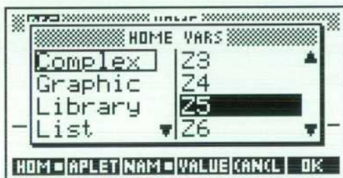
Fig. 30. Most variable values must be a specific type and several classes of variables contain exactly ten variables. For example, Z1 to Z9 are complex variables.
