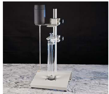
Hart's 2031A "Quick Stick" Immersion Freezer offers unmatched convenience and simplicity in forming the triple point of water ice mantle.
