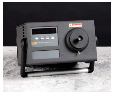
The 9133 includes a quick-attach fitting on the front bezel for dry air purging, which eliminates ice buildup on the target.
