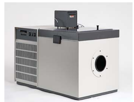
This Hart Model 7008-IR features a NIST-designed cone-shaped target.
