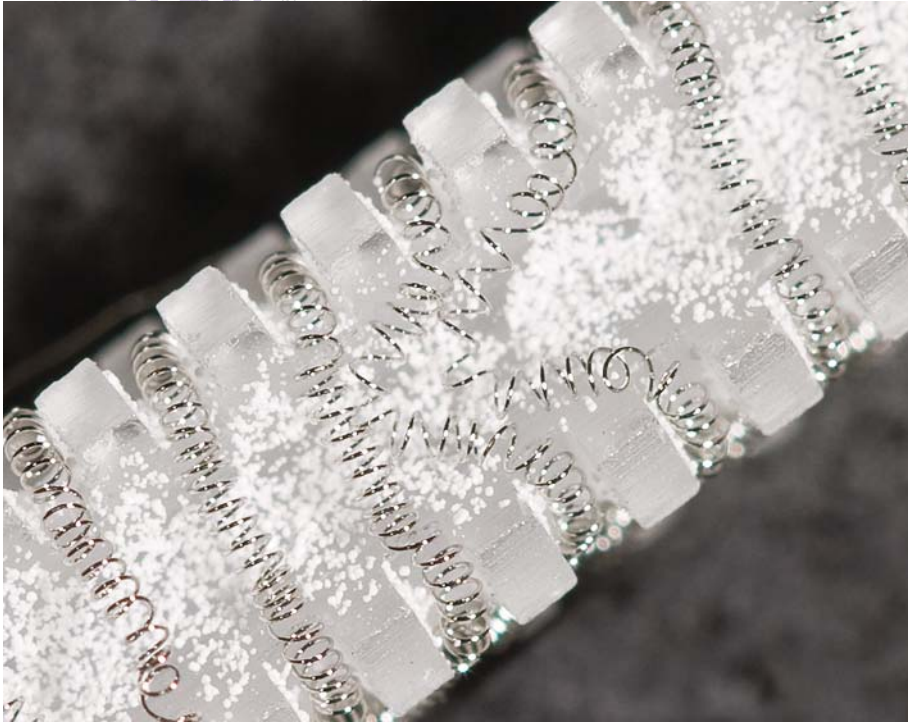
Damaged coils from a dropped sensor.
