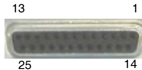
Fig. 2-8 Parallel Connector Pin Locations
