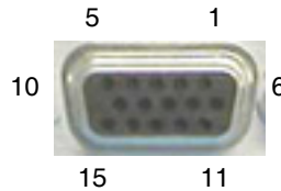
Fig. 2-9 VGA Monitor Output Pin Locations
