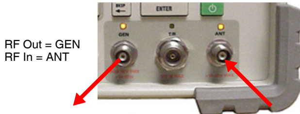
Fig. 3-29 GEN/ANT Two Port Duplex Test Setup
