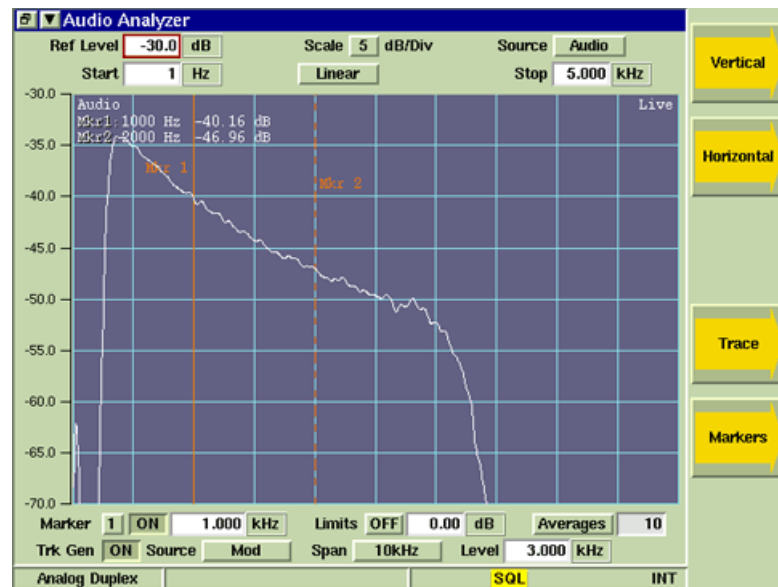
Fig. 6-51 Audio Analyzer - Rx Bandpass Sweep
