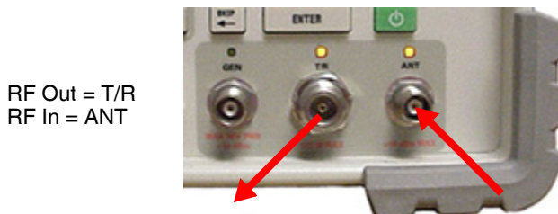
Fig. 3-31 TR/ANT Two Port Duplex Test Setup
