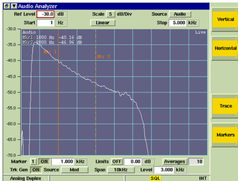
Fig. 8-8 Audio Analyzer - Rx Bandpass Sweep
