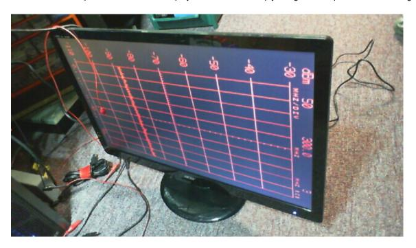
Inverting and combining sync and adjusting levels before going to GBS board was needed...but might not all be necessary...more testing to do...all this would fit easy in the space the CRT occupies.
