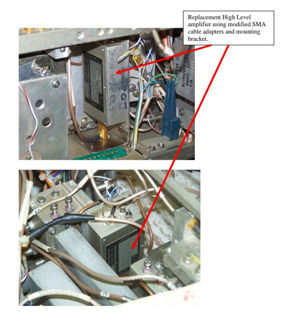
While the output of the Q-Bit 500-2 the IFR's output only goes from -33 dBm (5000 uV) to -13 dBm (50,000 uV) this 20 dB gain block provides enough RF output to jam a signal into almost any dead front end and do signal tracing with a spectrum analyzer or sensitive wide band oscilloscope. It probably is not enough power to radiate a test signal to a repeater.
