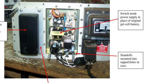
Plastic cover drilled to match original power supply holes.
