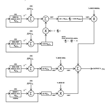
FIGURE 4-1: VOR SIGNAL GENERATOR BLOCK DIAGRAM
