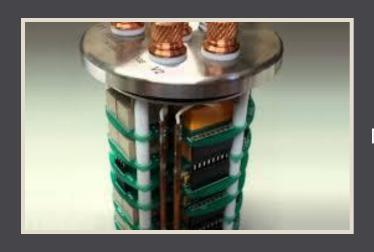
Operated via USB to PC Automatic, unattended measurements Reduction in hands-on staff time May be kept in a temperature-controlled resistor bath Decreased uncertainty contribution from TCR Stated accuracy: 0.01 ppm at 100  $\Omega$  Electrical switching-induced errors possible: noise, thermal EMFs (DC)
