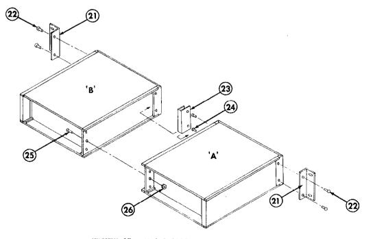
FIGURE 17. Model 1007 Dual Rack Mounting.
