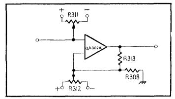
FIGURE 26. DC Offset Adjustment.
