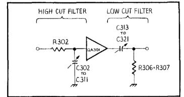
FIGURE 25. High-Low Cut Filter.
