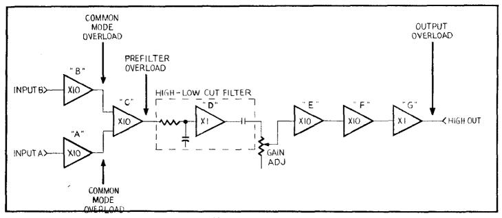
FIGURE 18. Overall Block Diagram.
