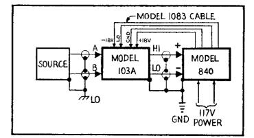
FIGURE 15. Use in System 84 Lockin Amplifier.
