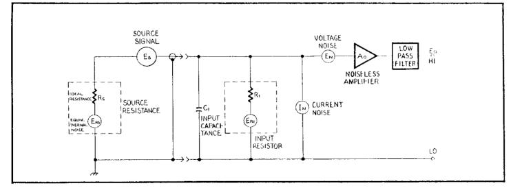
FIGURE 10. Equivalent Circuit For Noise Analysis.
