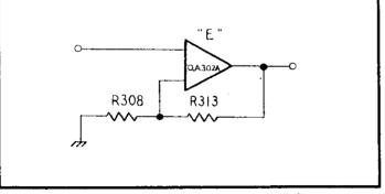
FIGURE 23. Non-inverting Stage "E".
