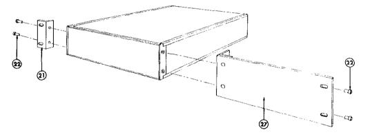
FIGURE 16. Model 2000 Rack Mounting.
