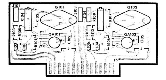
FIGURE 31. Component Layout, PC-261 (Model 1031A Regulator)
