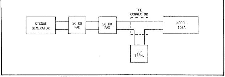
FIGURE 32. Test Set-up for Frequency Response Check.
