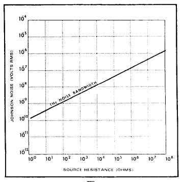
FIGURE 8. Johnson Noise/ WE Versus Source Resistance.
