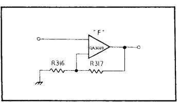
FIGURE 24. Non-inverting Stage "F".
