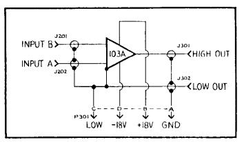
FIGURE 7b. Power Input Connection,
