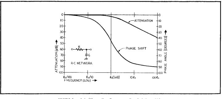
FIGURE 9. Gain/Phase Vs. Frequency For R-C Type Filter.
