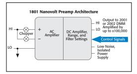
The Model 1801 can measure temperature differentials accurately using a variety of sensors, including type J, K, T, E, R, S, and B differential thermocouples. Users may also enter a specific  $\mu V/^{\circ}C$ value, making it possible to measure temperature using thermopiles. Thermistor measurements can be made by inputting a constant current to the sensor, then calculating temperature from the resulting  $\mu V/^{\circ}C$  output.
