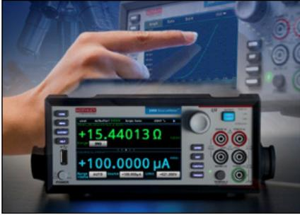
Figure 3. Modern SourceMeter SMU Instrument.
