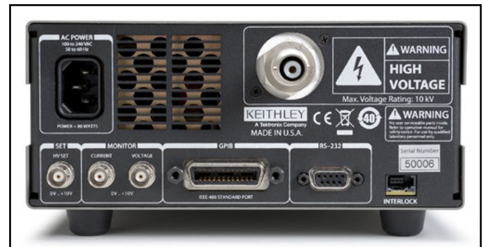
Model 2290-10 rear panel showing the IEEE-488 interface connector, RS-232 interface connector, high voltage output connector, analog control/output connectors, and interlock connector.
