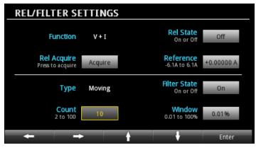
Figure 7. Series 2280S filter settings for low current measurements
