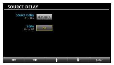
Figure 9. Series 2280S source delay settings for low current measurements
