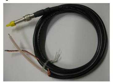
Figure 1: Model 2290-10 SHVUC male to unterminated cable
