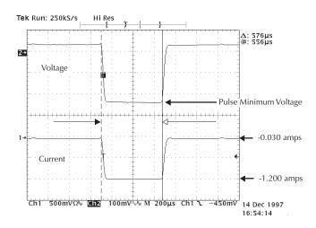
NOTE The simulated GSM phone current profile contained in Figure E-3 shows a standby current of 0.030A, a transmit current of 1.2A, and the pulse minimum voltage during the transmit frame.
