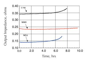
NOTE Figure E-4 shows electronic resistance for battery packs during a simulated GSM phone pulsed discharge from full charge to 5.5 volts.
