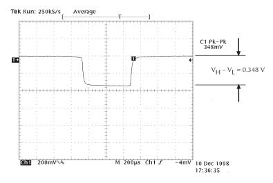
NOTE Figure E-6 shows the voltage drop during the transmit portion of the pulse of a GSM phone with the supplied Li ion.
