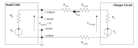
NOTE Figure 2-4 shows the preferred method for measuring current output of the charger circuit at a rated output voltage with the power supply operating in local sense mode.
