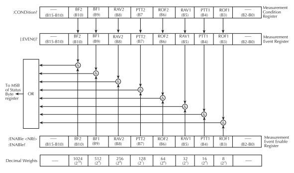
BF = Buffer Full RAV = Reading Available PTT = Pulse Trigger Timeout
