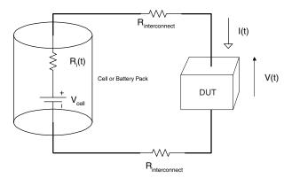
If  $R_{interconnect}$  is small compared to  $R_i(t)$  and  $R_i(t)$  is relatively constant during the length of the pulse,  $R_i(t) \sim R_i$ , then the voltage across the DUT may be expressed as:
