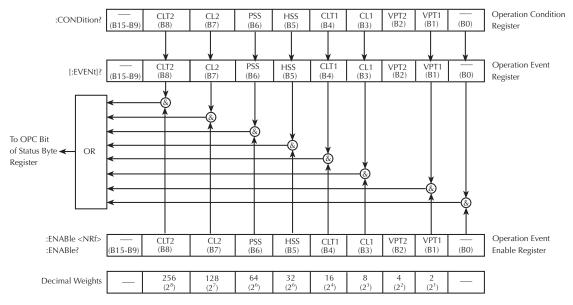
PSS = Power Supply Shutdown CLT = Current Limit Tripped
