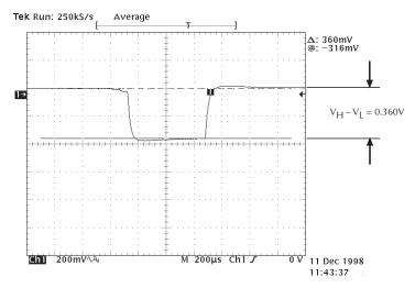
NOTE Figure E-7 contains the voltage drop during the transmit portion of the pulse of a GSM phone with the Model 2306 battery channel, output impedance set to  $0.24\Omega$ .
