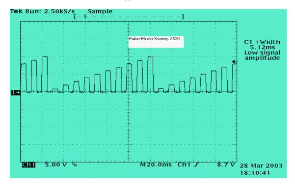
If selecting the Log sweep type, make sure you do not start the sweep from 0 Volts or 0 Amps as the logarithm of zero cannot be calculated.
