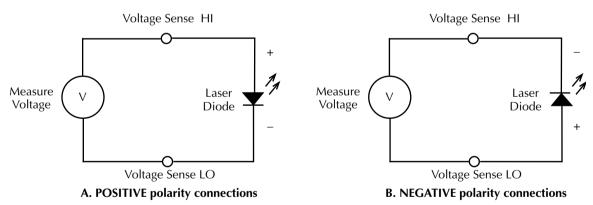
Note: Incorrect polarity setting will result in overflow voltage reading.
