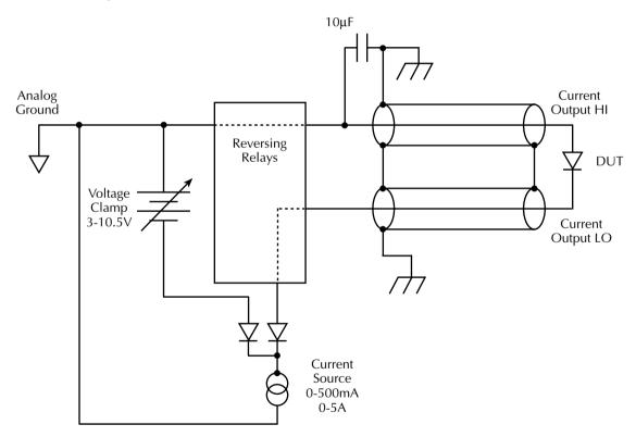
The voltage clamp circuit acts to limit maximum voltage as seen by the output of the pulse circuit. Since the clamp circuit is not directly across the laser diode, the voltage drop across the transmission line connected between the pulse source and the laser diode is not seen by the clamp circuit and cannot be regulated by the clamp. As a result, care must be taken to minimize the negative effects of the transmission line.
