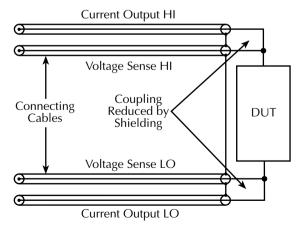
B. Coupling reduced by shielding.
