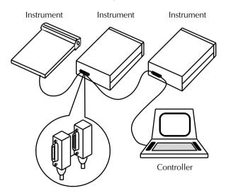
To avoid possible mechanical damage, stack no more than three connectors on any one unit.
