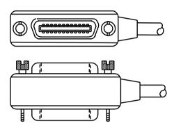
To allow many parallel connections to one instrument, stack the connectors. Two screws are located on each connector to ensure that connections remain secure. Figure 10-2 shows a typical connecting scheme for a multi-unit test system.
