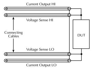
B. Correct: sense leads connected at DUT.
