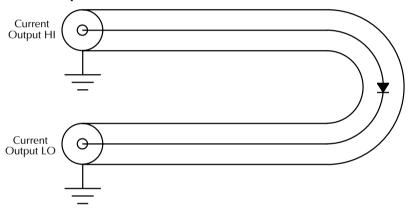
Figure F-13 **Compromised shield provides laser diode access**
