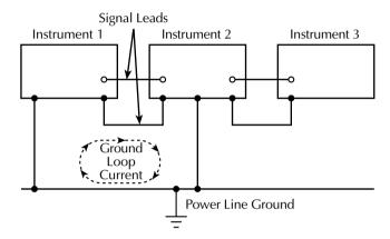
Figure F-19 Power line ground loops
