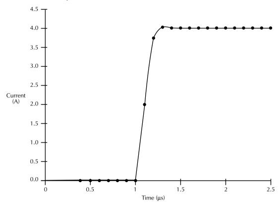
Figure F-3 **Rise time of 0.45A current pulse**
