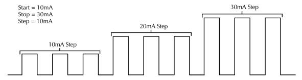
With filter count = 3, three delay-pulse cycles are performed at each sweep step.
