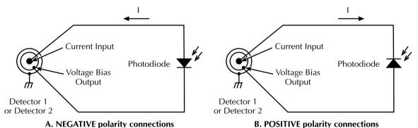
Note: Incorrect polarity setting will result in overflow current reading
