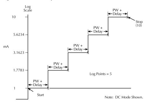
The programmable parameters for a log sweep include the start and stop levels and the number of measurement points for the sweep. The specified start, stop, and point parameters determine the logarithmic step size for the sweep. Step size for the sweep in Figure 7-2 is calculated as follows:
