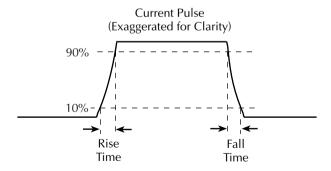
The rise and fall times of the current source pulse can be controlled with the :SOURce1:PULSe:TRANsition command, as covered in "SOURce subsystem," page 14-32. This command allows you to increase the rise time of the pulse. Increasing the rise time will help reduce overshoot and/or oscillations that could occur when long cables are used, or if poor connections are present in the test setup.
