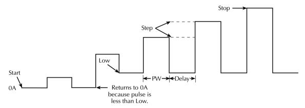
Figure 5-4 shows how various front panel programming parameters control various staircase sweep DC waveform aspects. These parameters are programmed by pressing the appropriate key:
