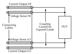
A. Coupling caused by exposed leads.
