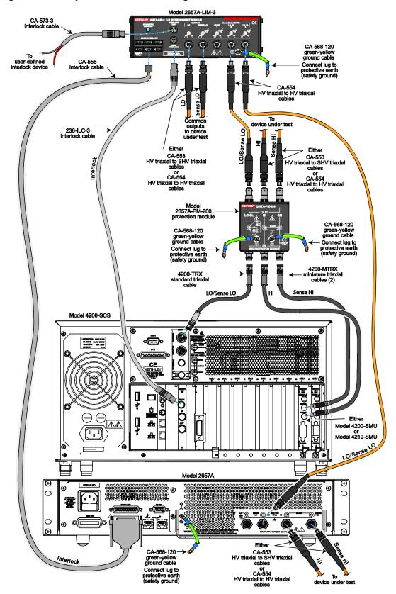
Figure 11: Test system connections using a Model 2657A and a Model 4200-SCS SMU
