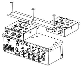
Figure 2: Mounting protection modules onto the Model 2657A-LIM-3
