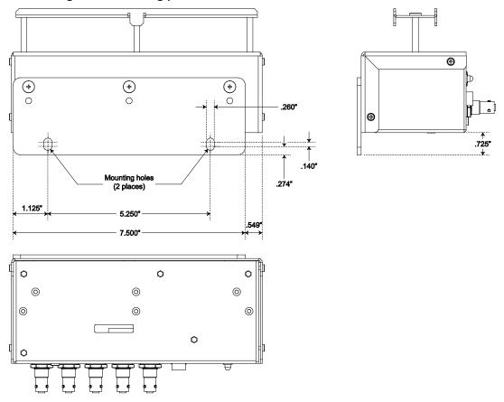
Figure 5: Mounting plate attached to the rear of the Model 2657-LIM-3
