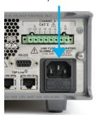
3. Connect the plug of the power cord to a grounded AC outlet.
