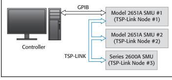
Figure 9: Communications setup for examples.
