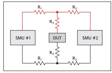
Figure 5: Model for test lead resistances.
