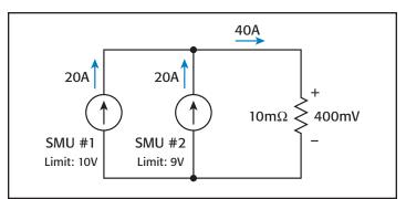
Figure 6: Example of two current source SMUs connected in parallel and functioning under normal operation.
