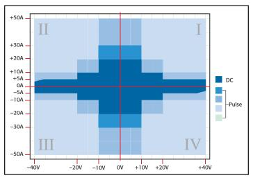
Figure 3: Power envelope for a single Model 2651A.
