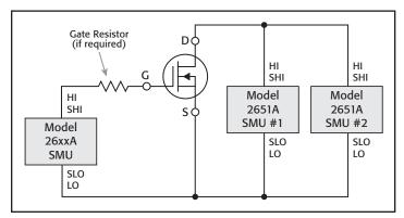
Figure 10: Connections for dual SMU Rds(on) sweep.
