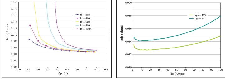
Figure 1: Example results after performing a pulsed Rds(on) current sweep (500µs pulse width and 0.01 NPLC) to test up to 100A on a power MOSFET device using two Model 2651A SourceMeter instruments connected in parallel.
