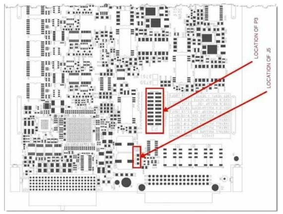
The connector labeled P3 contains all of the jumpers needed to configure digital I/O and VEXT1, VEXT2. The connector labeled J5 contains a single jumper option that configures the backplane relays. See the following table for individual jumper locations and effects.
