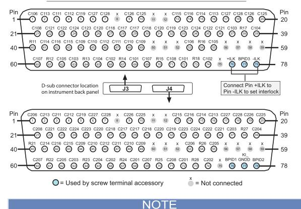
The pinouts in the previous figure represent the pin connections that are made when the Model 3732-ST-R screw terminal is attached to the Model 3732 J3 and J4 connectors. If the Model 3732-ST-R is not attached, you must connect the pins with the same name together externally; they are not connected on the Model 3732 card for this mode.
