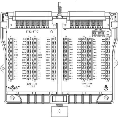
Figure 40: Model 3732-ST-C screw terminal assembly circuit board
