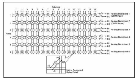
Figure 30: Schematic of the Model 3730
