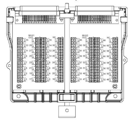
Figure 27: Model 3724 screw terminal assembly circuit board
