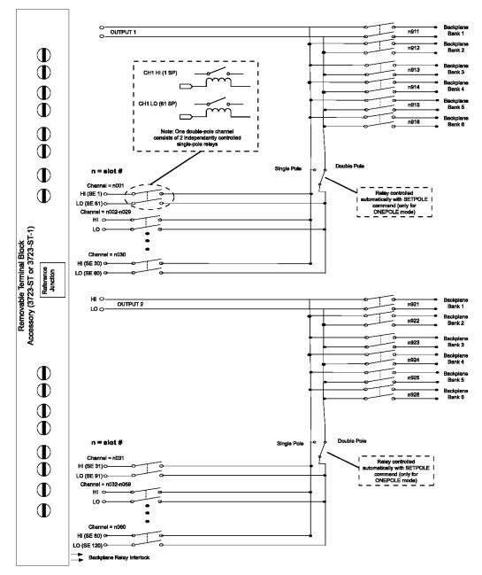
The following figure provides a switching schematic for the Model 3723 in single-pole mode.
