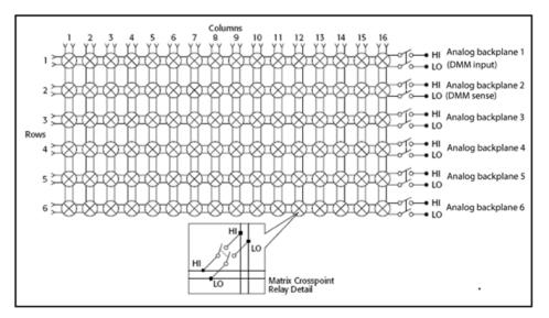
Figure 34: Model 3731 simplified crosspoint relay schematic
