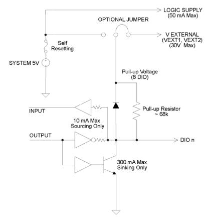
The figure shows a simplified schematic for one bit of a digital I/O channel. Each I/O bit has an optional pullup resistor in parallel with a diode that is used to clamp flyback voltages from inductive devices like electro-mechanical relays. However, when the optional jumper is removed, both the pullup resistor and diode are removed from the circuit. The pullup resistor is considered "weak" and can easily be overdriven by the external circuit.
