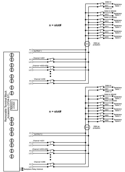
The next Figure is a diagram of the screw terminal assembly:
