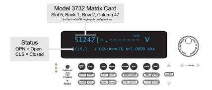
Also, you can now press the DISPLAY button to navigate from the main screen to a screen showing the closed channels on the system. If there are more channels than fit on one screen, use the navigation wheel to scroll through the channels. Press the DISPLAY button to navigate back through the menus to the main screen.
