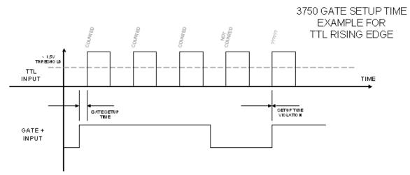
MINIMUM GATE INPUT SETUP TIME:
