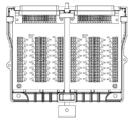
Figure 6: Model 3720 screw terminal assembly circuit board
