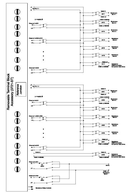
Figure 9: Schematic of the Model 3721 in two-pole mode
