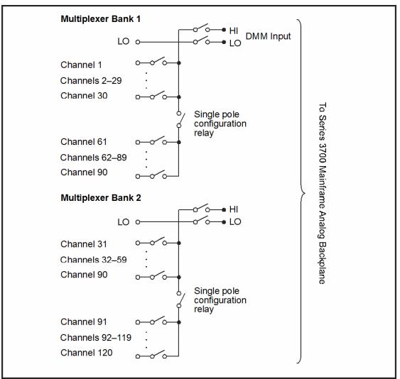
Figure 21: Schematic: Model 3723 in one-pole mode
