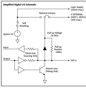
Figure 2. Simplified I/O schematic
