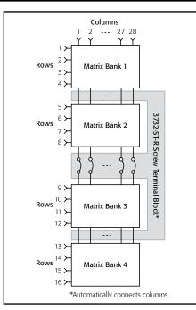
Single 16×28 (1-wire) matrix configuration using one Model 3732-ST-R screw terminal block SWITCHING AND CONTROL
