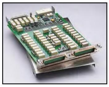
The Model 3721 offers two independent banks of  $1\times20$  two-pole multiplexers that are ideal for general purpose switching, including temperature measurements. The two banks can automatically be connected to the Series 3700 mainframe backplane and optional DMM through the analog backplane connection relays. This connection allows the mainframe to reconfigure the Model 3721 as a single  $1\times40$  two-pole multiplexer or to enable card-to-card expansion for even larger configurations.
