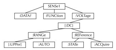
A command summary table is a way of documenting SCPI commands, but it does not show complete command names. A complete command is formed by joining the components. For example, the complete: STATe command in the example is:
