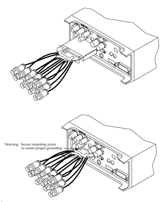
Figure 2-10 Scanner card installation
