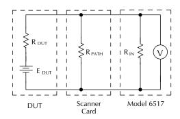
R<sub>DUT</sub> = Source Resistance of DUT
