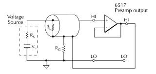
R<sub>S</sub> = Source resistance R<sub>L</sub> = Leakage resistance
