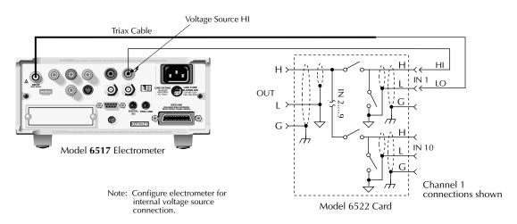
Figure 4-5 Connections for input isolation
