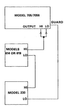
Figure 6. Model 7056 Isolation Test In Model 705
