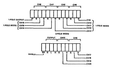
Figure 3. 1-Pole Mode Channel Numbering
