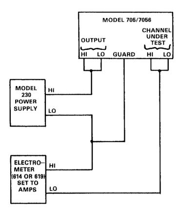
Figure 8. Channel Isolation Test Set Up
