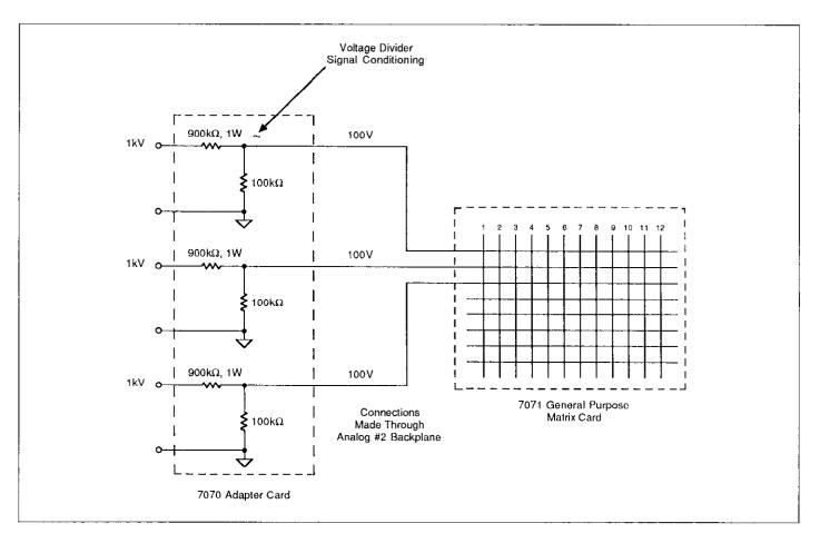
Figure 3-19. Signal Conditioning Example
