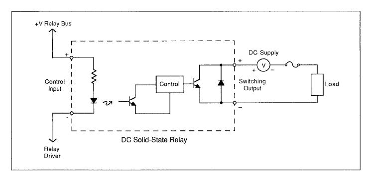
Figure 3-12. Typical DC Solid-state Relay
