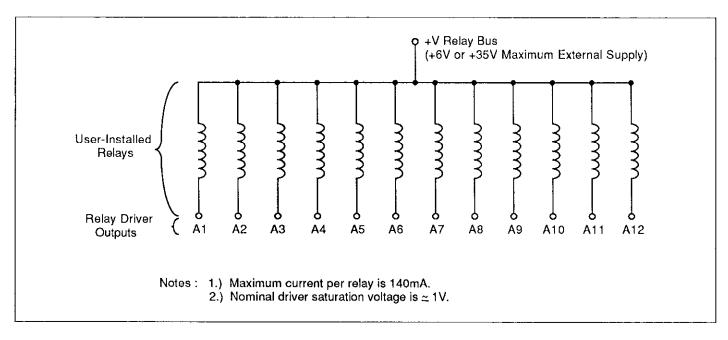
Figure 2-10. Typical Relay Coil Connections (Row A Shown)
