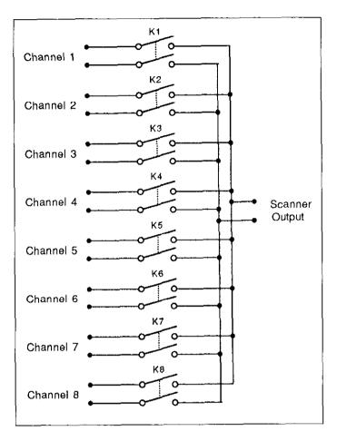
Figure 3-2. 8-Input, 2-Pole Relay Scanner
