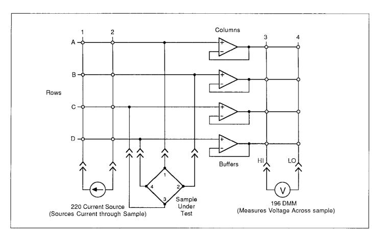
Figure 3-9. Typical High-Resistivity Test System
