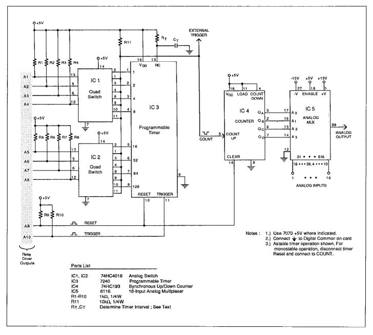
Figure 3-16. High-Speed Analog Multiplexer with Control Circuit
