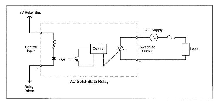
Figure 3-13. Typical AC Solid-state Relay
