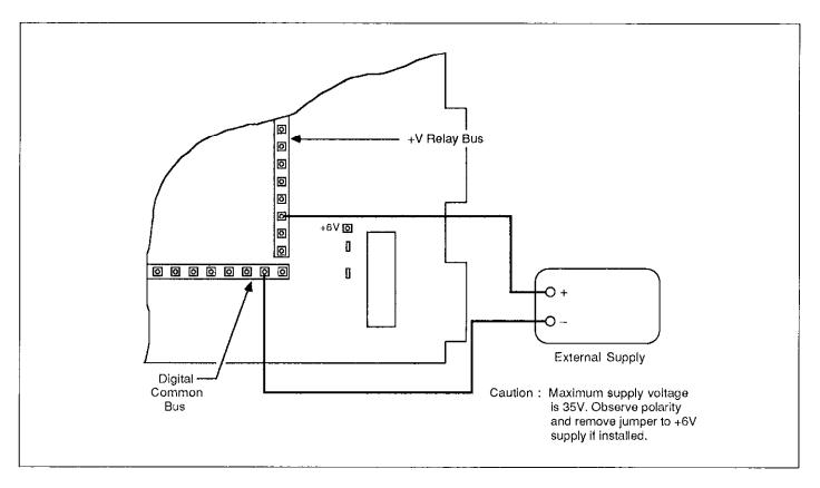
Figure 2-8. External Supply Connections
