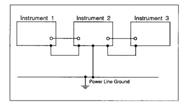
Figure 2-16. Eliminating Ground Loops
