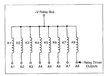
Figure 3-3. Scanner Relay Coil Wiring
