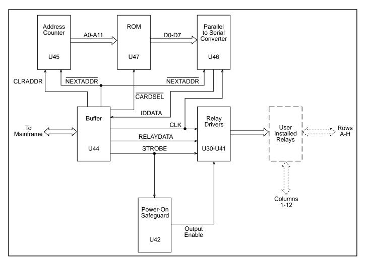
Figure 4-3. Model 7070 Block Diagram
