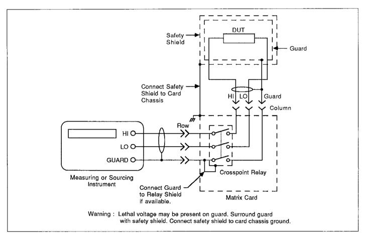
Figure 2-19. Typical Guarded Connections
