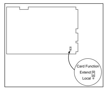
Figure 2-2. Extend Function Jumper Selection
