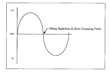
Figure 3-11. Zero-crossing Switching
