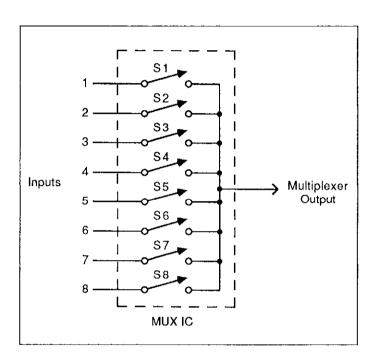
Figure 3-15. Typical Multiplexer IC
