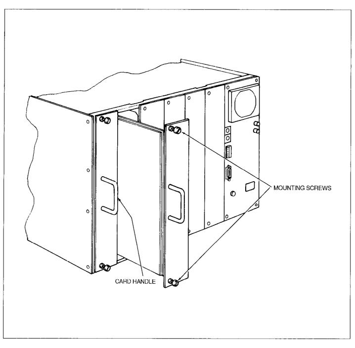
Figure 2-5. Model 7070 Installation
