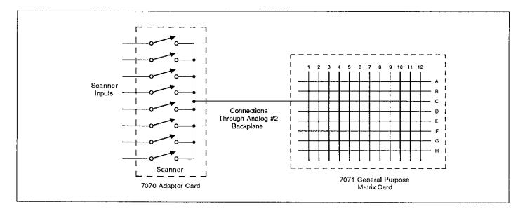
Figure 3-18. Adding a Scanner to a Switching Matrix
