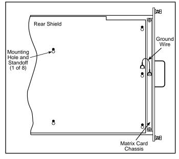
Figure 4-1. Removing the Rear Shield
