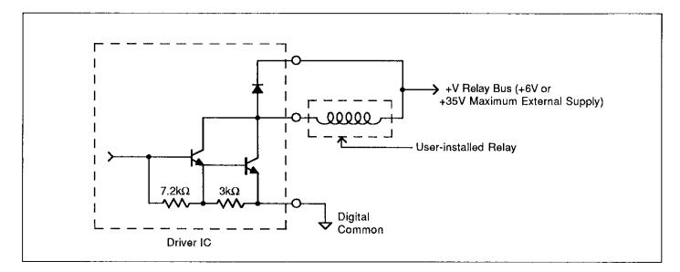
Figure 2-9. Typical Relay Driver Output
