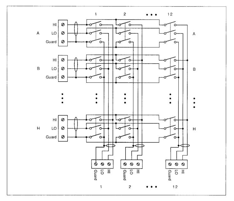
Figure 2-11. Relay Matrix Wiring
