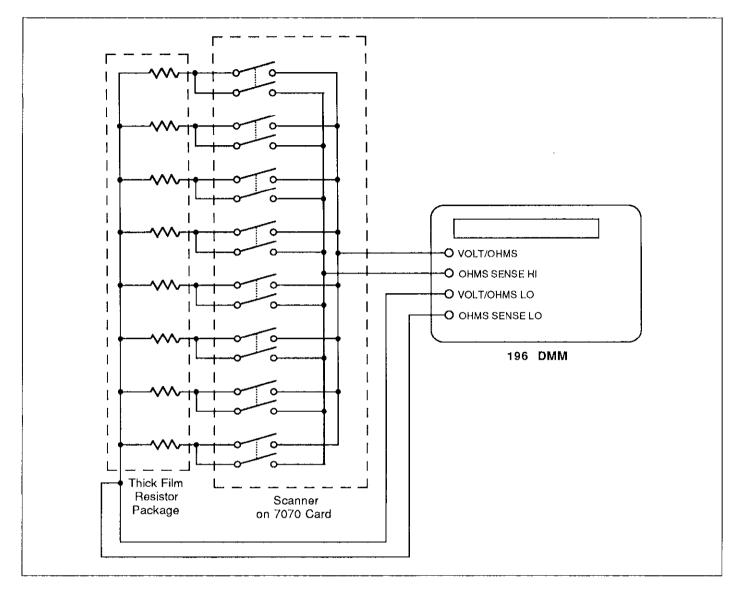
Figure 3-5. Testing Thick Film Resistor with a Scanner
