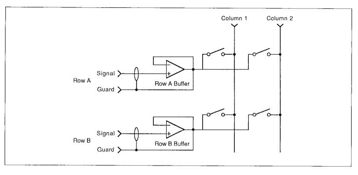
Figure 3-7. Buffer Configuration
