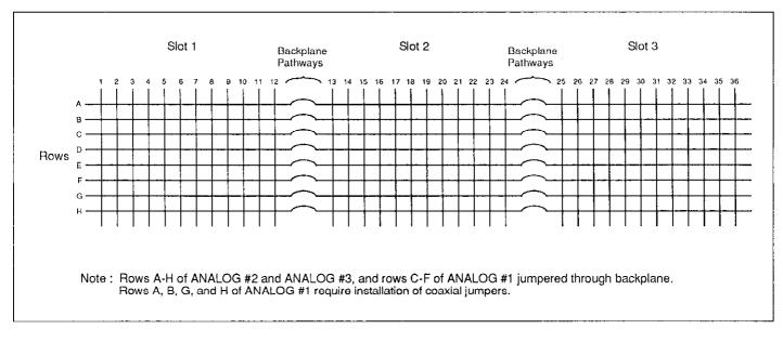
Figure 2-13. Connecting Three Cards for 8  $\times$  36 Matrix
