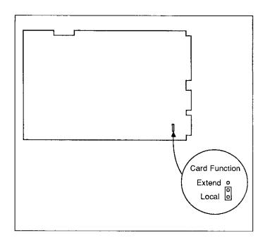
Figure 2-6. LOCAL Function Jumper Position
