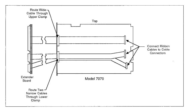
Figure 2-3. Ribbon Cable Connections
