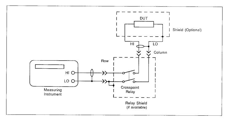
Figure 2-17. Shielding Example
