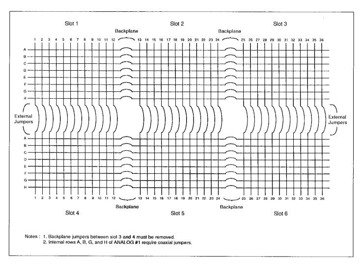
Figure 2-14. 16  $\times$  36 Matrix Constructed by External Jumporing
