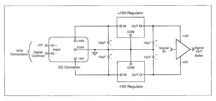
Figure 3-8. DC Converter Used to Power Buffer ICs
