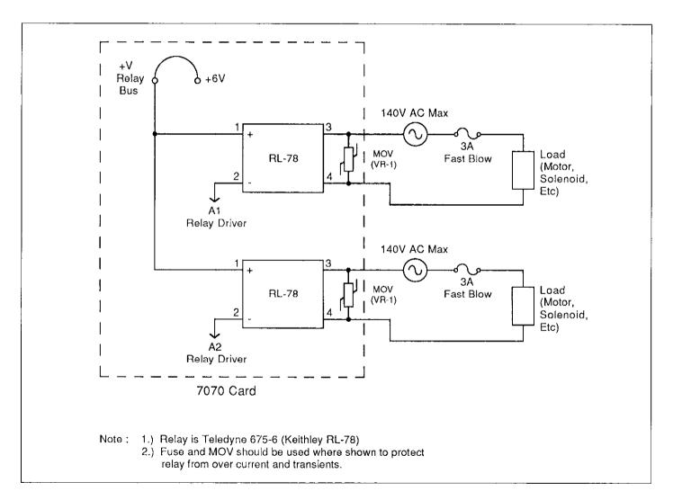
Figure 3-14. Typical Solid-state Relay Application
