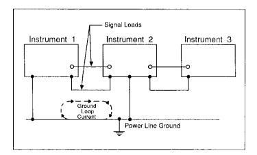
Figure 2-15. Power Line Ground Loops
