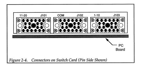
The connector on the switch card will mate to either a connector (Model 7169-KIT) or to an optional mass terminated cable (Model 7169-MTC-10).
