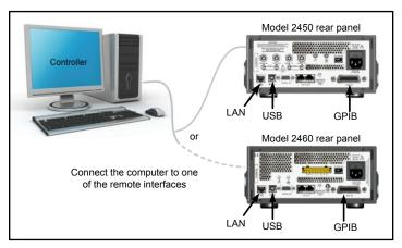
Figure 4. Model 2450 or Model 2460 SourceMeter SMU Instrument remote interface connections.
