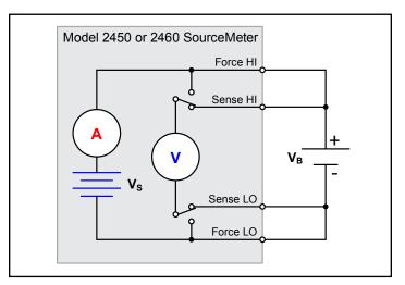
Figure 3. Connecting the Model 2450 or Model 2460 SourceMeter SMU Instrument to the battery.
