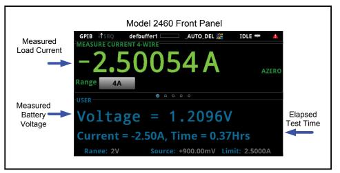
Figure 6. Model 2450 or Model 2460 SourceMeter SMU Instrument displaying the load current, battery voltage, and elapsed test time while discharging a D cell battery.
