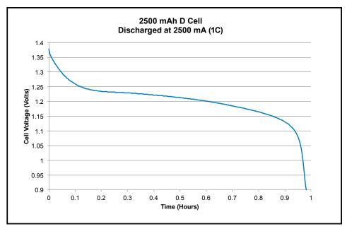
Figure 5. Discharge characteristics of 2500mAh D cell battery.
