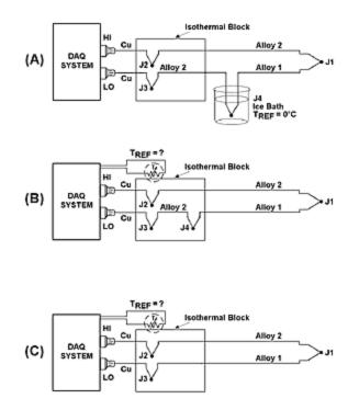
In Figure 2B, we move the reference junction (J4) onto the isothermal block, with the result that the instrument terminals and the reference junction are now at the same temperature. This temperature can be read with a sensor that does not require a reference junction, such as a thermistor or semiconductor temperature sensor.
