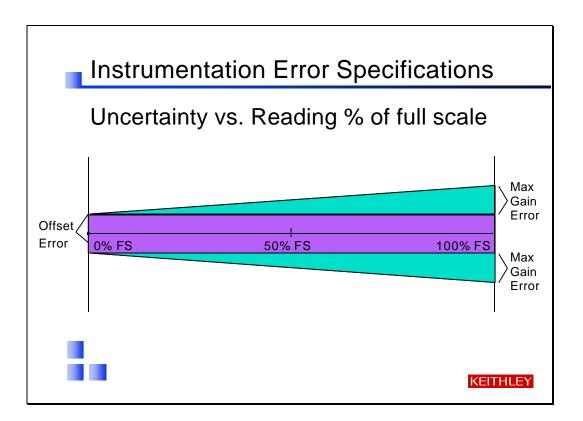
Instrument specifications can be stated in a variety of ways: parts per million (ppm), percent or counts. (ppm is used instead of percent when the magnitude of the numbers are small; 10,000 ppm = 1%)
