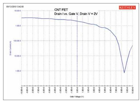
Figure 5. Drain current vs. gate voltage of CNT FET
