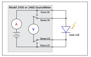
Figure 5. Connections from the SourceMeter instrument to the solar cell or panel.
