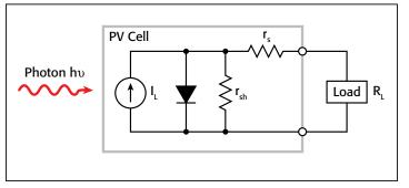
Figure 2. Idealized equivalent circuit of a photovoltaic cell.
