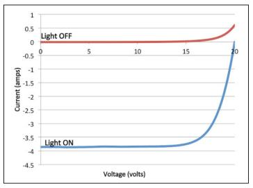
Figure 8. Solar cell I-V sweeps generated by Model 2460.
