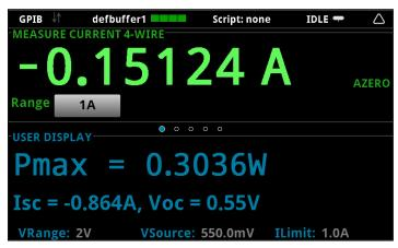
Figure 9. The 2450 display indicates maximum power ( $P_{max}$ ), short circuit current ( $I_{sc}$ ), and open circuit voltage ( $V_{oc}$ ).
