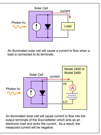
Figure 4. A SourceMeter instrument acts as an electronic load when connected to an illuminated PV cell.
