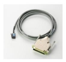
The Model CA-558 cable connects the safety interlock circuit of a Series 26xxA SourceMeter to the safety interlock switch of the Model 8010 High Power Device Test Fixture that contains the device under test. To use the cable, plug one end of the cable into the interlock connector on the test fixture, and connect the other end of the cable into the INTERLOCK connector on the rear panel of the instrument.
