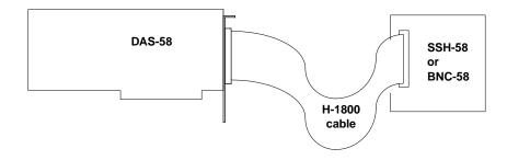
Figure 1. Cabling the DAS-58 to an SSH-58 or BNC-58
