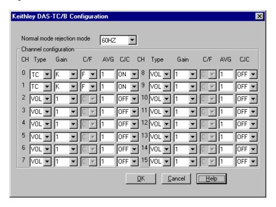
In LabVIEW, do not wire any values to the upper or lower limit terminals of the VIs. When not wired, a value of zero is provided to the DriverLINX driver, which will cause the board to be operated according to the settings in the DriverLINX Configuration Panel (above).
