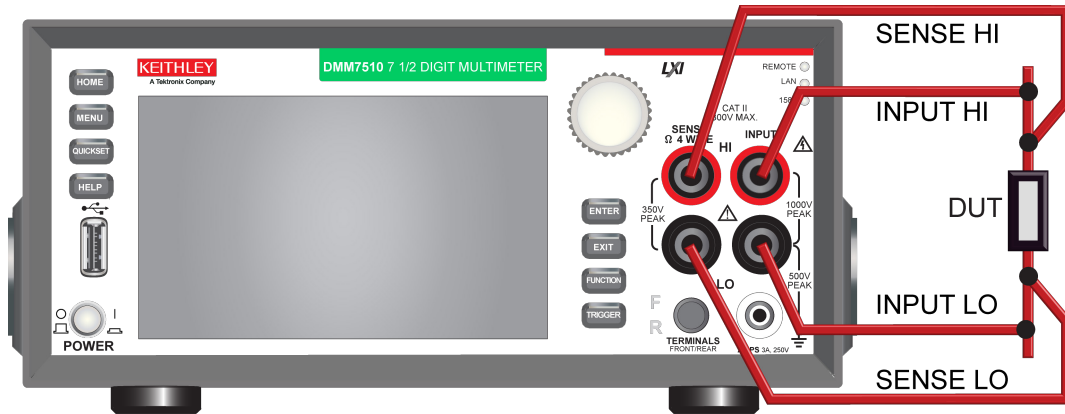
Figure 71: Model DMM7510 front-panel 4-wire remote sense connections
