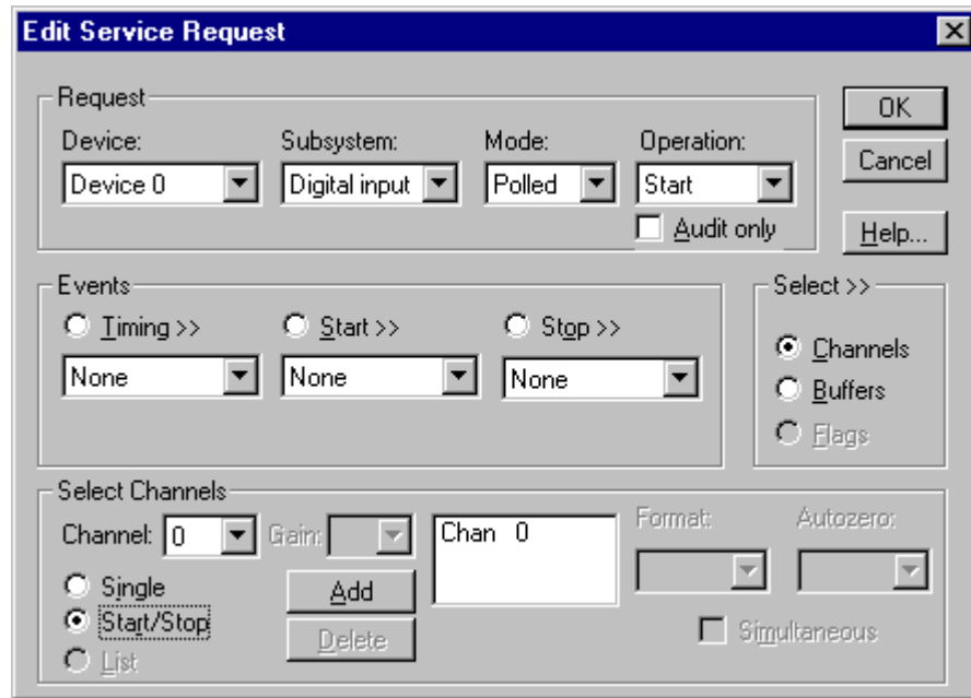
How to set up the KPCI-3108 Series for sampling on a consecutive range of channels.
