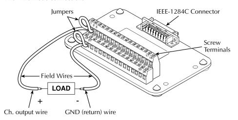
Figure 3 Example of a two-wire mode connection
