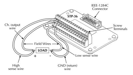
Figure 5 Signal descriptions for "Analog" I/O connector pins and screw-terminals
