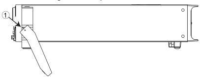
2. After you align the arrows, pull the ends of the handle (1) away from the case.
