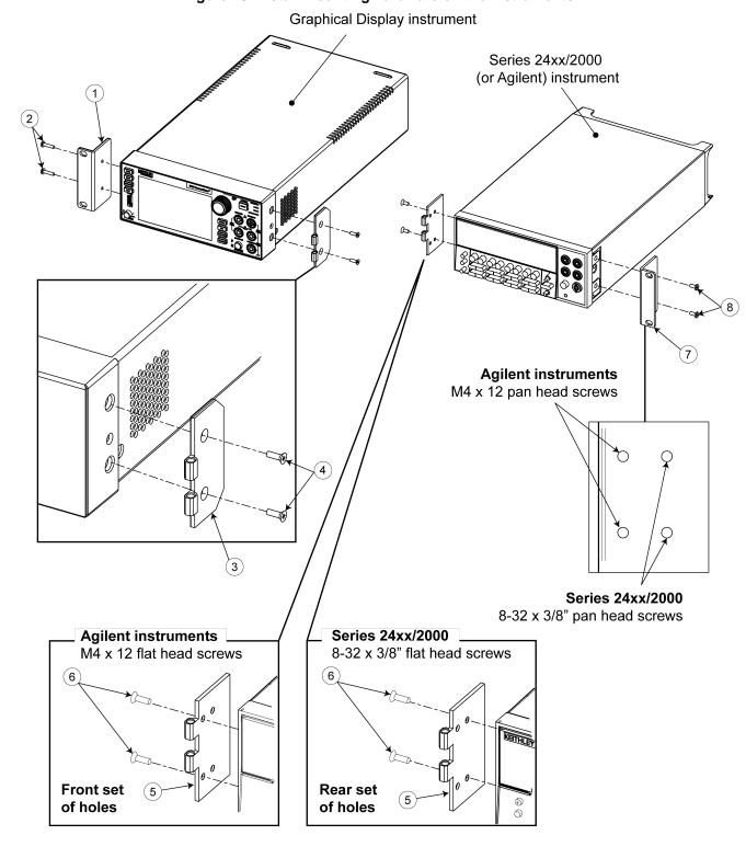
Figure 10: Install mounting hardware on the instruments
