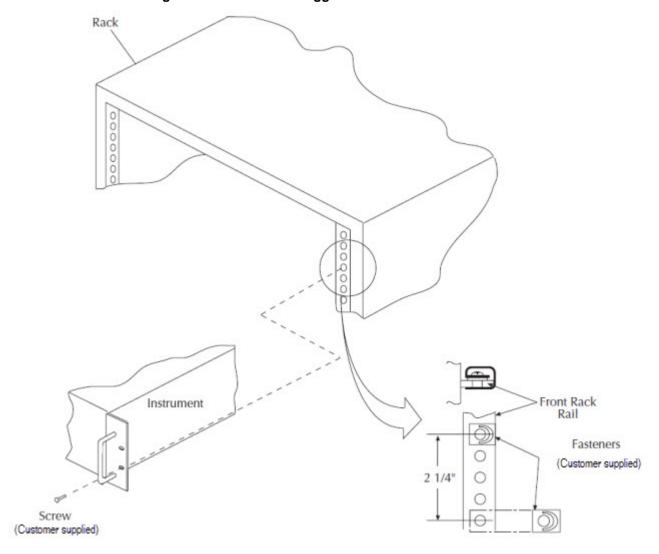
Figure 2: Model 2290-5 suggested rack fastener installation
