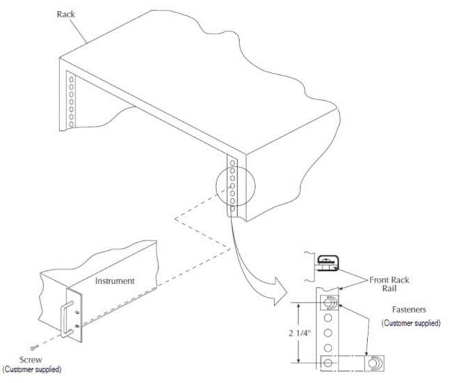
Figure 2: Model 2290-5 suggested single rack fastener installation
