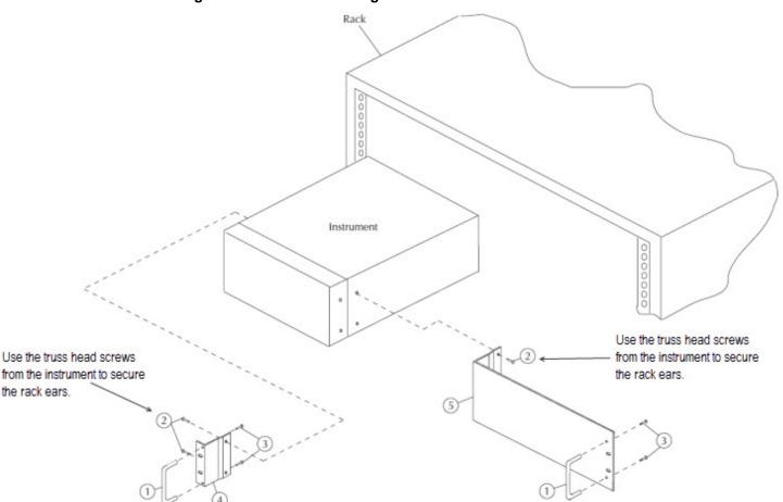
Figure 1: Model 2290-10 single rack mount kit installation
