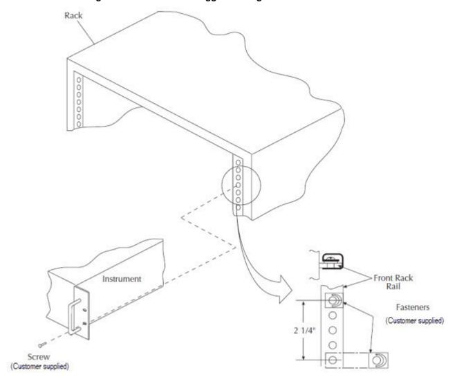
Figure 2: Model 2290-10 suggested single rack fastener installation
