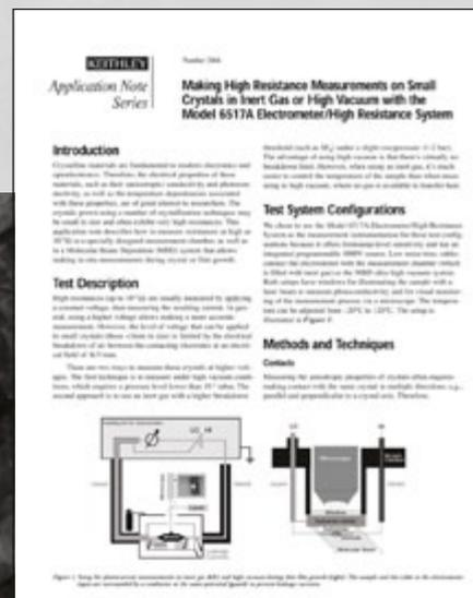
In this system configured for photocurrent measurements, the sample and the cable to the electrometer input are surrounded by a conductor at the same potential (guard) to prevent leakage currents.
