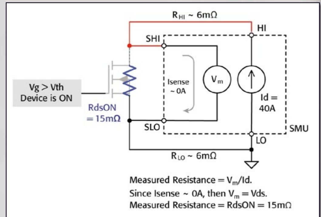
Use separate test leads to connect the device to the instrument's sense terminals. In this way, the voltage measured is only that across the device. The resulting resistance measurement will be a true measurement of the DUT resistance.
