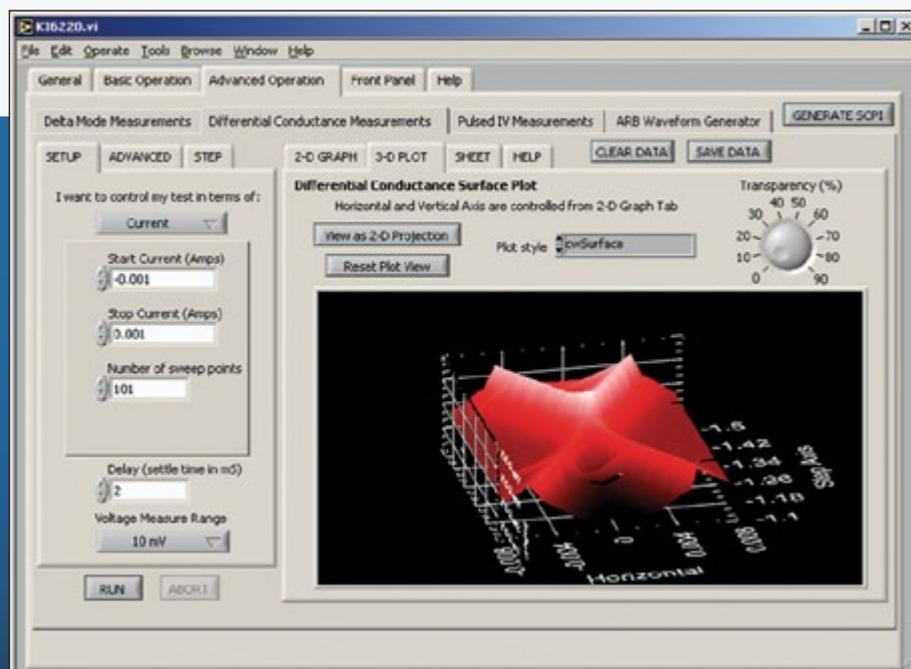
The 622X/2182A combination makes it simple to perform, analyze, and display differential conductance measurements.
