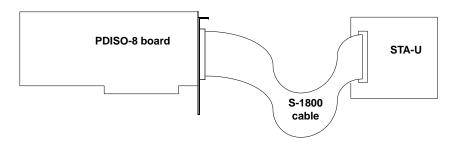
Figure 1. Attaching a PDISO-8 Board to an STA-U
