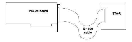
Figure 1. Attaching a PIO-24 Board to an STA-U
