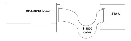
Figure 1. Attaching a DDA-08/16 Board to an STA-U
