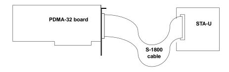
Figure 1. Connecting a PDMA-32 Board to an STA-U
