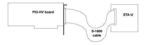
Figure 1. Connecting a PIO-HV Board to an STA-U
